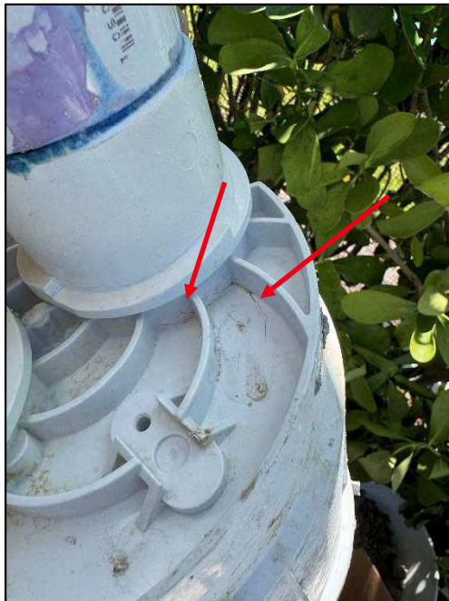
Crack found in the pool skimmer body
